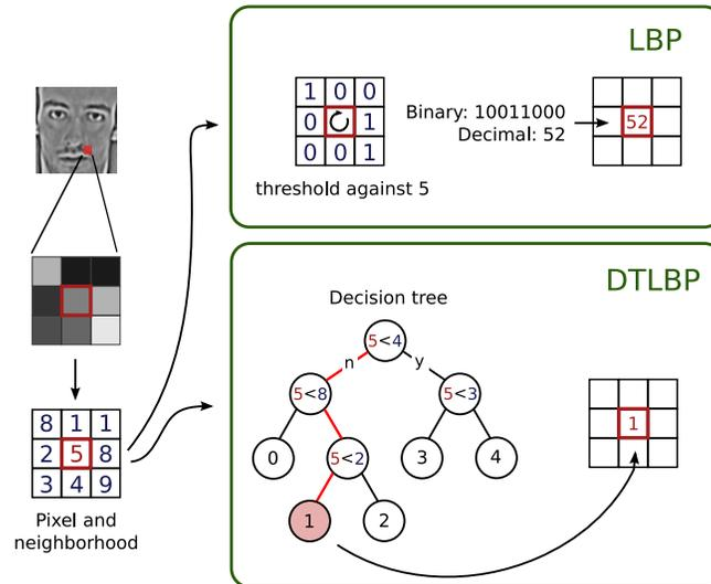
Fig. 2: The LBP operator versus the DT-LBP operator.
